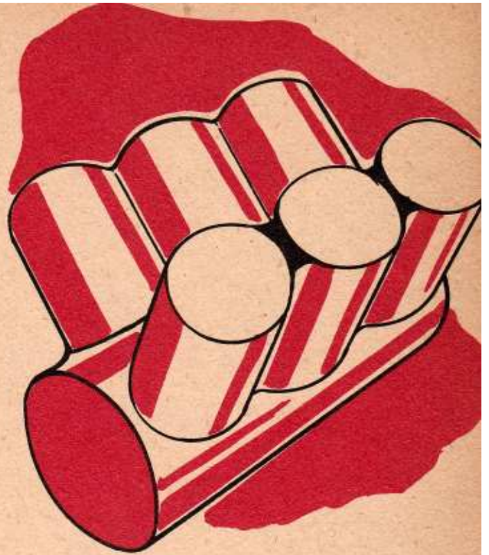
Cylinders arranged in a V-formation in a six-cylinder engine.
